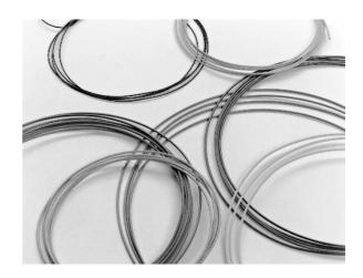
SPEC 44 wire has a dual wall construction which combines the outstanding physical and electrical characteristics of radiation crosslinked polyalkene with the excellent mechanical and chemical properties of radiation cross-linked polyvinylidene fluoride (PVDF).
